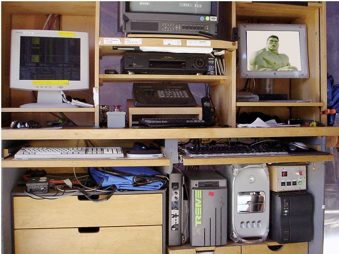
This is ILM's motion control Mac workstation. The Xtreme DDR (left of the G4) stores the motion control sequence, which then gets composited with the CG elements on the Mac in After Effects. Photo: Scott C. Smith, ILM
